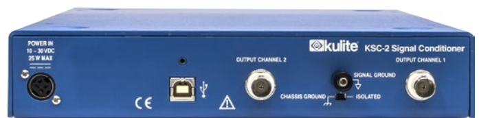
KSC-2 Signal Conditioner Rear View
