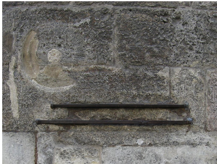
Official Viennese linen ell and drapery ell length standards embedded in the cathedral wall
