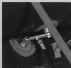
Dual SS inflation system to assure full redundancy.
