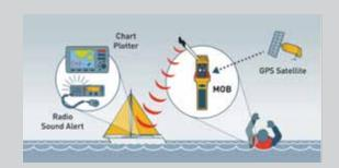
The MOB1 is intended to be installed within the life-jacket and will activate automatically on inflation, sending the first alert within 15 seconds. The integrated strobe light ensures maximum visibility in low light conditions. The MOB1 communicates with the vessel you have been separated from and other vessels in the vicinity (up to 5 miles range dependent on conditions).
