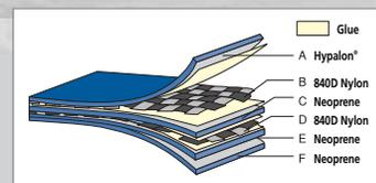
Double layer (840 denier each) nylon core fabric; reinforced with Hypalon® and Neoprene
