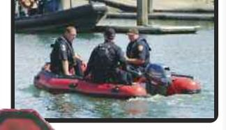
Designed originally as rapid response boats for fire departments and rescue units, these unique aluminum roll up floors with an innovative hinge system and non-skid panels can perform a variety of functions. They are easy to store or carry and can be set up in minutes. The main air chambers are equipped with over pressure relief valves so they can be inflated either by compressed air bottles or the standard equipment foot pump.
