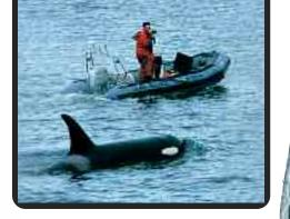
SU boats are made with an additional heavy-duty layer of 840-denier nylon Achilles CSM fabric in a two-ply technique which results in a fabric even stronger than a single base fabric of equal thickness. A number of commercial grade features such as recessed valves and a full-length, protective wear patch combine to make these boats the right choice for the toughest marine uses. SPORT UTILITY SERIES
