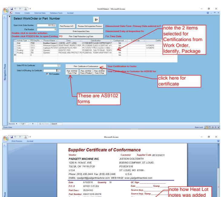
Drawing No. 68A311230-2007B Shipper\_ Work Order No. RevIECO E DCN M033363, SPECO 0001 Process Supplier/Processor Name Description Specification C17200 BERYLLIUM COPPE BAR PER ASTM-B 196, CON HT (TH04) HE AT LOT NO. 0001530878 (24185), DATED 10/21/2014 Beryllium Copper 2.00 Rd x 6 2.00 RD. x 6 FT. LONG Ft. C17200 ASTM-B196, Cond. HT (TH04) FARMERS COPPER LTD results of See PO Module and line items CHROME PLUS INTERNATIO processing added and how notes can be added PS 13101VTYPE II, CLASS 3
