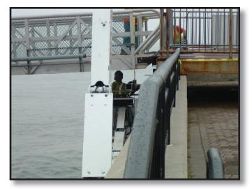
**Extra Agility** is a standard feature on the UB50 and UB60 models. These units offer a hydraulic activated fourth boom which extends the working range to include travel between bridge girders to get a close-up look at the back side. When the boom is placed perpendicular to the third boom, it is capable of placing an inspection 7' (2.1m) above the third boom on the model UB50, 9'9" (3.0 m) on the model UB60
