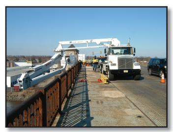
**Maneuverability** Two rotating turrets are provided, one at the pedestal (T-1) affording 155° of rotation and one at the end of the first boom (T-2) with up to 360° rotation. In the deployed position, T-2 has 224° rotation to provide more agility to thread through tight truss work and maneuver around underbridge supports, providing easier access to more underbridge area.
