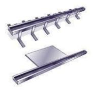
The channel is notched on the top of one end to receive the insert washers. Both ends of the channel are closed with endcaps welded in place.
