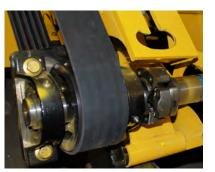
A clutchless PTO system allows the cutter to be engaged without using a traditional slip clutch or idler pulley and without sliding the engine. The system is simple to maintain — once under the shield, belt changes are easily accomplished without the use of tools.
