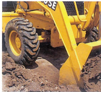
Available mechanical-front-wheel-drive provides extra power and traction to heap the bucket regardless of what's underfoot. Its limited-slip design automatically transfers up to 80 percent of available power to the wheel with the best traction.
