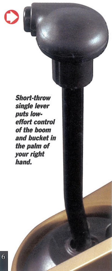
Transmission disconnect switch diverts full engine power to the hydraulics for faster loading.
