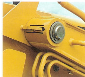
Bucket level indicator is within your line-of-sight. Nearby automatic return-to-dig switch is well-protected, yet easily accessible. Hydraulic self-leveling and float are also standard.
