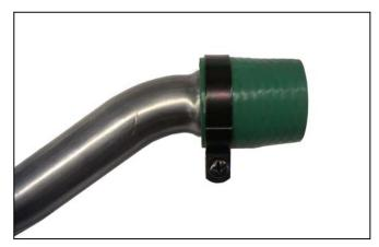
Now you can tighten the forward clamp on the pipe seal tightly against the pipe stinger tip larger diameter part for a good seal.
