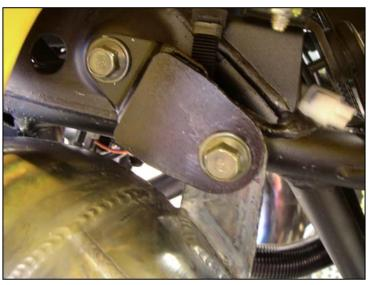
that the stinger (pipe outlet) is held  $\underline{above}$  the choke lever (plunger) back at the carbs. Then just push the pipe up on the cylinder spud making sure that it is straight and parallel to the spud axis.
