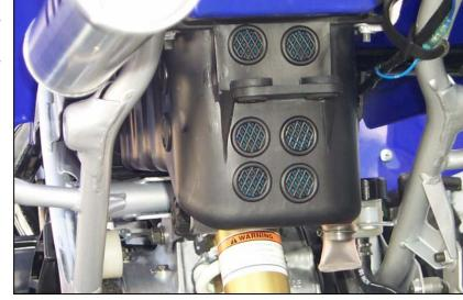
over flash on the edge of the holes might prevent the Uni-Vents from seating properly. Then just push the filtered vents in the holes. They just snap in.
