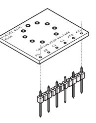
Align the noval socket (provided with the kit) with the hole pattern on the top of the board, insert pins through holes and solder.
