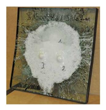
A thin and lightweight ballistic glazing solution, only 23 mm thick
