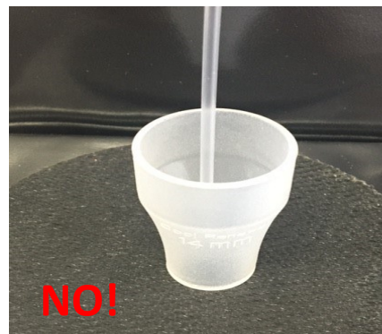
Incorrect– 90° Spray Angle
