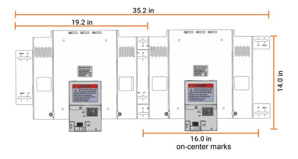
Wall Area Required for Number of Batteries with 16-Inch Wall Mount Brackets
