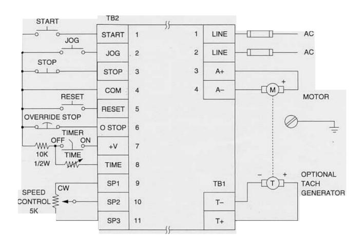
WARNING: TB1 TERMINALS T+ AND T- ARE AT RECTIFIED AC LINE VOLTAGE AT ALL TIMES POWER IS APPLIED TO THE DRIVE WHETHER OR NOT THE DRIVE IS TURNING THE MOTOR.
