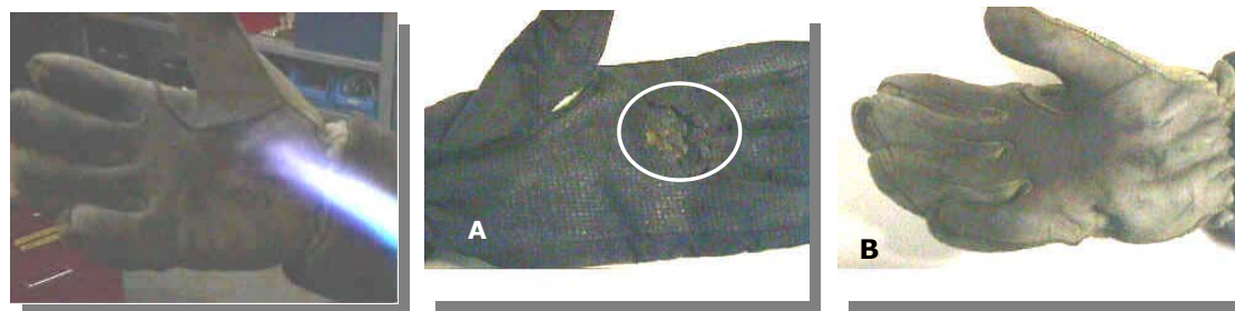
Figure VI.9 Gasburner tests conducted at the Dusseldorf firebrigade (Germany),
