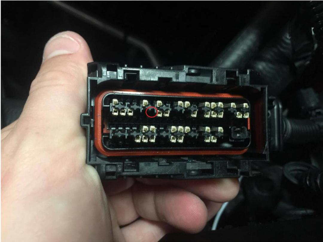
8. Zip tie the wire bunch if necessary and replace covers, and prepare to reattach harness connector to the PCM
