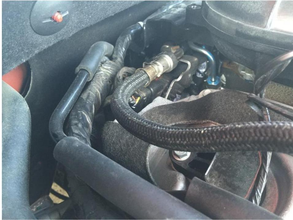
In the picture above find where the factory flexible fuel line meets the hardline towards the firewall at the passenger side of the engine.
