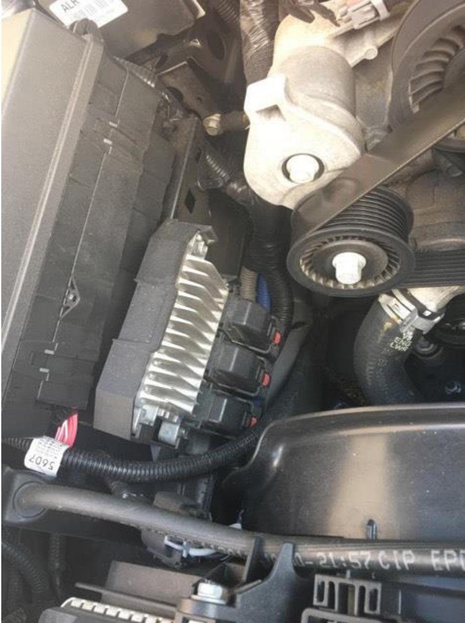
6. Unplug the blue connector and disassemble plastic cover to expose the wires, remove front blue trim ring as well to expose the terminal side of the connector
