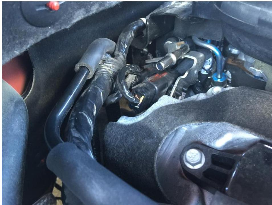
Using a 3/8 fuel line disconnect tool, disconnect the flexible line to make room for your flex sensor kit. The sensor will snap onto the flex line side and the billet adapter will screw over the hardline (refer to 1<sup>st</sup> picture above if you need help)
