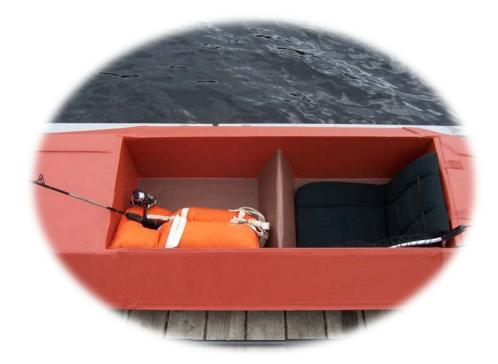
Notice the Velcro strips around the top of the stern bulkhead that secure the electric motor mount on top of the stern.
