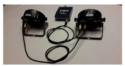
For Best DMX fixture/device control, power up AC, address and daisy chain all units <u>BEFORE</u> connecting to the CNF DMX Lighting Control Module. Then power up the module.
