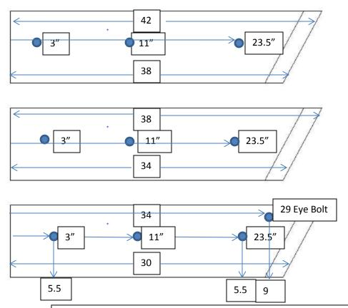
Planer boards are made from wood stair treds purchased at home depot or lowes. 3 pieces of 28" inch(heavy gauge) rebar connect the boards by measuring from the end of each board and drilling a hole at the 3,11 and 23.5 inch marks. An eye bolt is attached at the 29inch mark 9inches from the bottom. These boards will handle the worst the bay has to offer.
