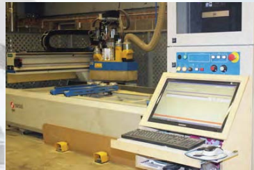
In-house CNC wood cutting for Upholstery production, ensuring accuracy and repeatability
