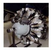
The legendary R-2800 that powered the Marauder and many other superb aircraft (see the list below) is widely considered to be one of the finest piston aircraft engines ever developed. It was a two-row, 18-cylinder, air-cooled radial design displacing 2,804 cubic inches (46 liters), with a bore of 5.75 inches (146 mm) and a stroke of 6 inches (152 mm).
