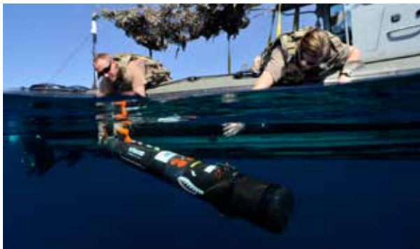
This is a Hydroid MK18 Mod 2 Swordfish is deployed to survey the ocean floor. Photo by Blake Midnight.
