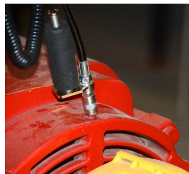
Figure 3: Examples of an acoustic lubrication delivery system. Note: An ultrasound instrument and a grease gun can also suffice.
