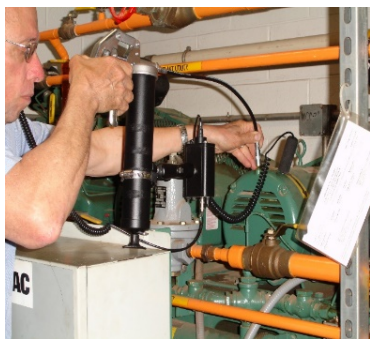
Figure 3: Examples of an acoustic lubrication delivery system. Note: An ultrasound instrument and a grease gun can also suffice.
