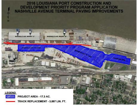
The Nashville Avenue Terminal Paving *Improvements* project consists of the demolition of 17.3 acres existing concrete pavers, construction of heavy-duty concrete paving in place of the pavers, demolition and replacement of 3,887 linear feet of existing rail track along perimeter of the area to be paved, installation of underground utilities. removal of the existing drainage system and installation of a new drainage system, removal of existing
