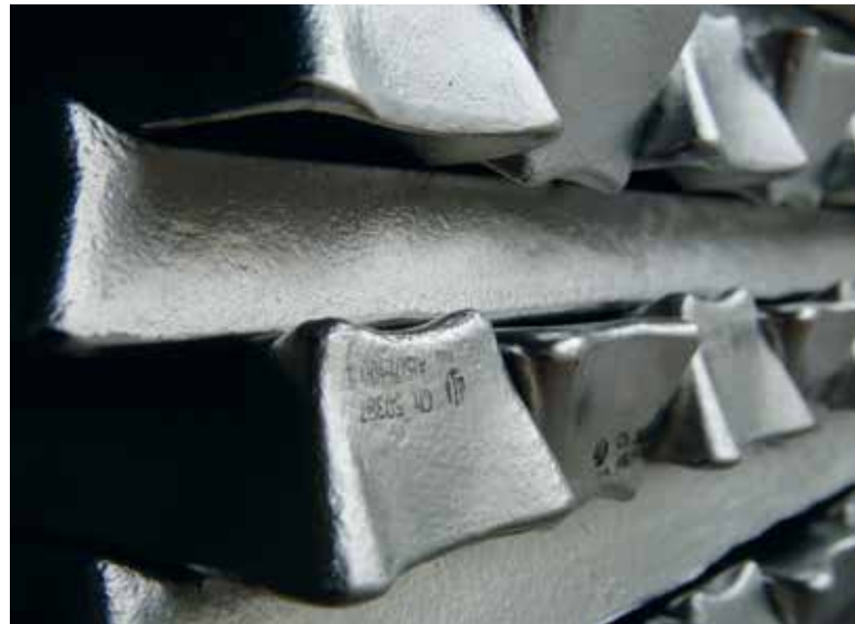
Aluminium foundry alloys are produced as continuous cast or mold-cast ingots for cast products.
