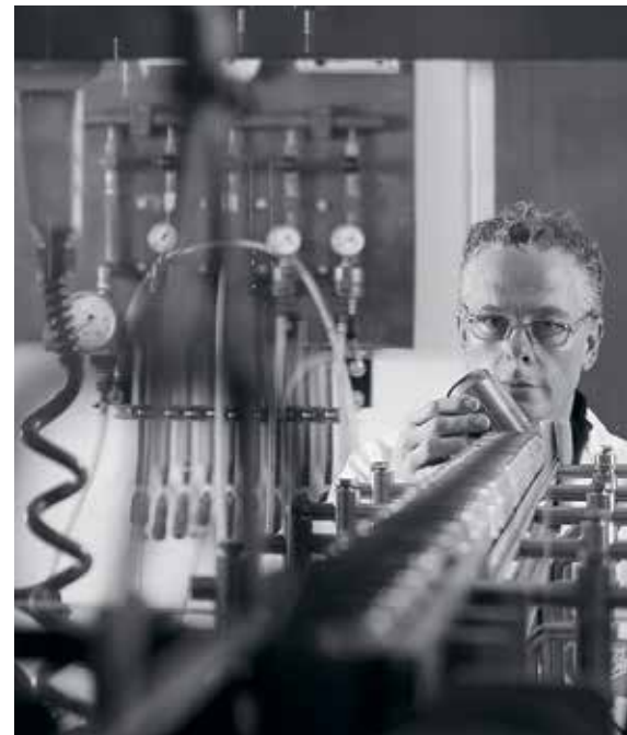
Ball’s test canning line is able to simulate production conditions as realistically as possible.
