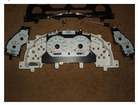
Remove the Torx T-10 screw that holds the speedometer/tachometer assembly in the cluster and remove the speedometer/tachometer assembly.
