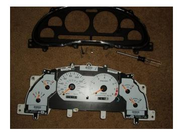
Unplug and place aside the dual minor gauge assemblies from either side of the speedometer/tachometer assembly.
