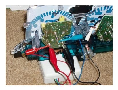
Using a flat-bladed screwdriver, turn the tach calibration potentiometer knob until the needle points to the RPM point being generated by the calibration signal generator.
