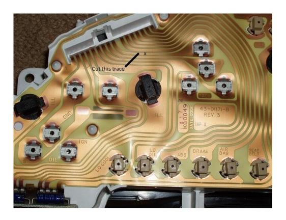
After you have cut the trace, the tachometer will operate in V6 mode. However, the tachometer will not be properly calibrated for a V6 since it was calibrated for a V8. You can calibrate the tachometer by providing it with power and a reference signal that you know corresponds with a known V6 RPM, and adjust the tachometer calibration potentiometer until the needle points to that RPM.
