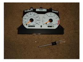
6. Flip the speedometer/tachometer pair upside down on top of the cluster so the unit is not resting on the needles. You can now identify the three 5mm screws that hold the cluster and you can see the cable that runs from the speedometer to the odometer motor. Since someone had remeoved the odometer motor from this cluster, the motor and cable are missing from my pictures.
