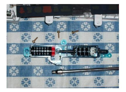
8. Swap the odometers, replace the 3 screws and connect the odometer motor cable in the same way you took it off.
