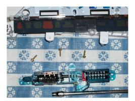
Here is the front view of the odometer:
