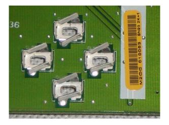
Once the pins have been bent away from the holes, enlarge the holes by carefully enlarging them until a 3/16" drill bit will pass through them. If you drill the holes out, drill from the PCB side, but drilling can tear up the female connector base. Some people run a 3/16" drill bit backwards in a drill press. I recommend a small cone shaped burr in a Dremel tool to widen the holes until the drill bit will fit through the hole. See the burr photo on page 6.
