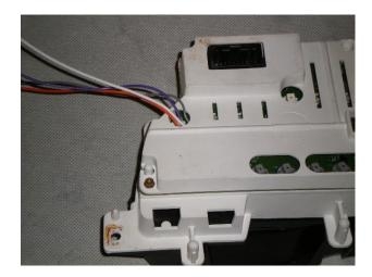
Move the cluster with the Upgrade Box now attached to the cockpit of the car. Connect the red wire to the switched power of your choice and connect the black wire to your good chassis ground. Connect the blue wire to the wire you ran from the oil pressure sensor on the engine or to the White/Red OEM oil pressure signal wire from the sensor if you are using the OEM wire.
