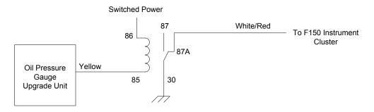
If you did not replace the F150 OEM oil pressure sensor with the Autometer sensor, you can simply leave the yellow wire from the upgrade unit unhooked.
