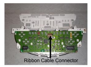
Unplug the ribbon cable connector and remove the Printed Circuit Board (PCB) from the back of the cluster. Locate the male pins on the back of the oil pressure gauge (bottom left gauge when viewed from the back of the cluster.)
