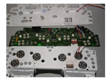
You should not have to take plastic front cover off of the cluster, but if you do, be sure not to lose the little coupler that connects the odometer reset rod to its switch on the PCB. Also, don't lose the rod itself.
