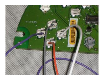
Plug the gray wire all the way down onto the top oil pressure gauge pin. Plug the white wire all the way down onto the right pin, plug the purple wire onto the left pin and plug the orange wire onto the bottom pin. Carefully slide the PCB down the wires until the pin holes are close to the ends of the wires.
