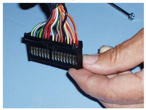
Once the connector is open, you can then push down on the black plastic tab in the hole in the connector pin to release the pin. While pushing down on the black plastic tab, pull back on the wire and the pin will come out.
