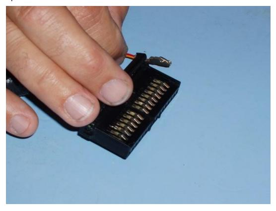
To put a pin back in, just slide the pin into the connector body until it clicks into place.
