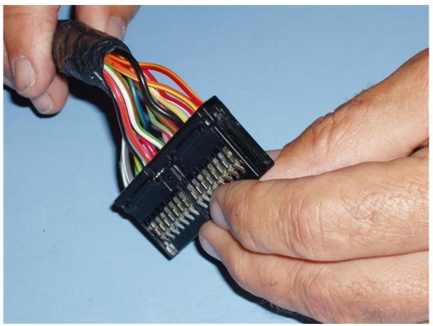
The two pins you need to swap are pins 14 and 15 of connector C250. C250 is the right hand connector when viewing the cluster from its rear, and the two pins you need to swap are the second and third pins from the right of the connector when viewed from the back of the cluster. On my 96/97 harness, pin 14 (Temp gauge signal) is a red wire with a white strip. Pin 15 (GND) is an orange wire with a yellow stripe.
