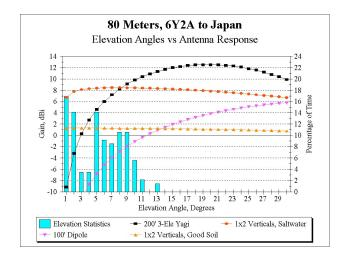
Overlaid on the take off angles is the elevationplane analysis of "standard" 80-meter antennas. Lets look at the 80-meter dipole at 100' (pink with inverted triangles). By most standards, this is a very good antenna. But you can clearly see there is little gain at the low angles.
