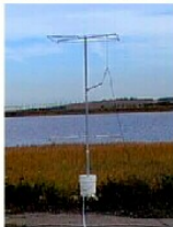
A single band ZR for 20 meters that is 6' tall. The feed is less than 50 ohms and is matched with a simple hairpin.
