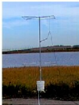
A single band ZR for 20 meters that is 6' tall. The feed is less than 50 ohms and is matched with a simple hairpin.
