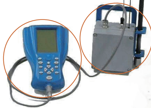
Central acquisition unit CAU (measure of the driving depth)
