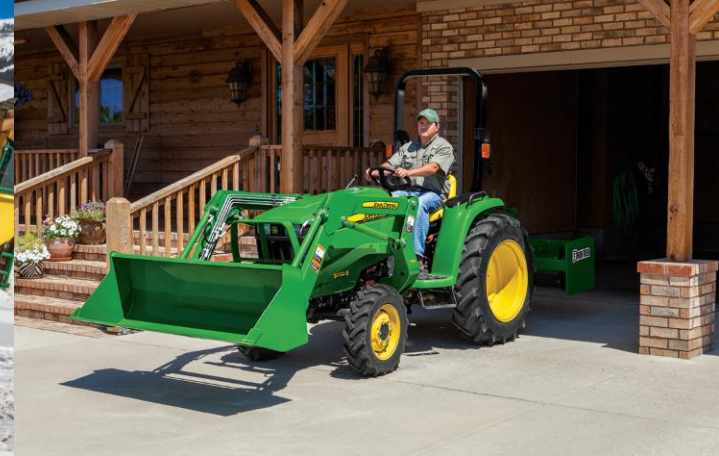
ASAE Roll Over Protection System (ROPS) enhances safety, and folds to fit easily in low doorways.
