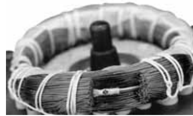
Fig. 24 PTC sensor incorporated in winding
