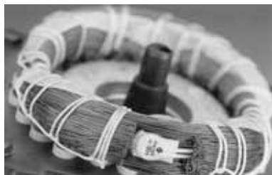
Fig. 26 Thermal switch incorporated in winding
