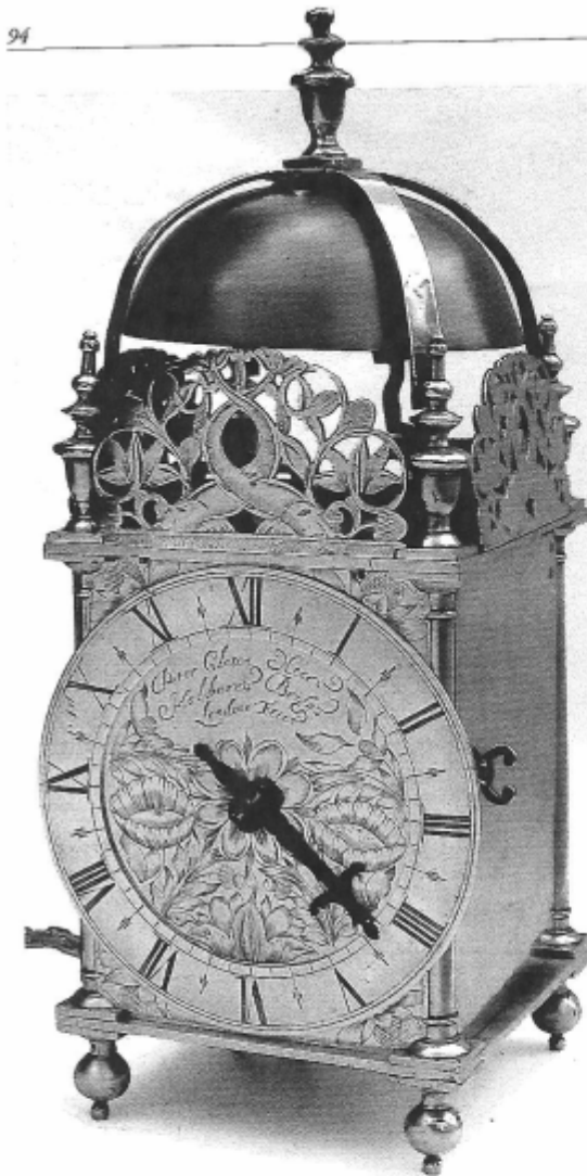
Fig 8.5 Originally a balance-wheel clock by Peter Closon, converted later to verge pendulum. Late features are: matchstick flower half-hour markers, dolphin frets, late pattern finials but grander and taller than usual. Date 1650s. (Photograph: John Robey)
