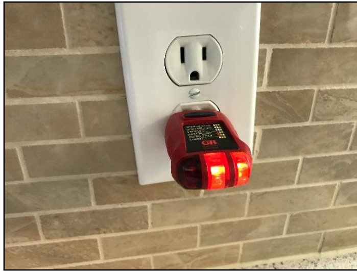
22. No GFCI/GFI (Ground Fault Circuit...
