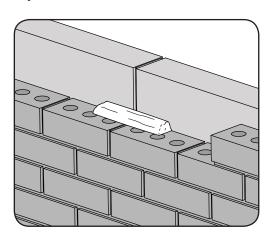
2. Lay a small bed of mortar along the back edge of the course directly below where the swift brick will sit.
