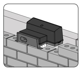
3. Bed the product into position, ensuring that the front edge is flush to the brickwork and the central drainage hole aligns with the perp joint of the course below.
