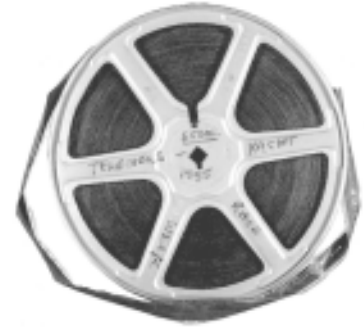
Fig. 13 Shrunken, embrittled 16mm acetate motion picture film.
