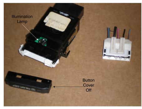
Remove the illumination lamp and then the white button slider and its springs:
