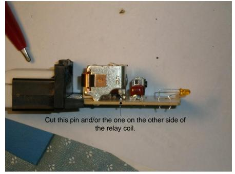
Here is the top view of the modified circuit board:
