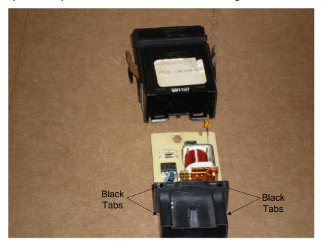
Remove the LED current limiting resistor and short the two indicated pads:
