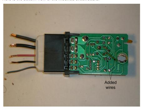
Reassemble the modified module without the button cap, slider, springs, illumination bulb or removed resistor. Cover the bulb socket with electrical tape:
