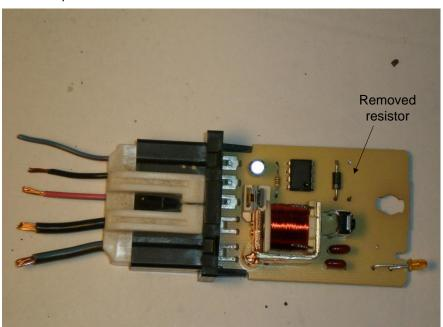
Here is the bottom view of the modified circuit board:
