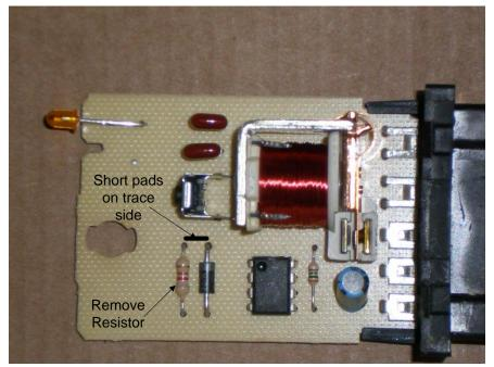
Cut one or both of the relay coil pins to disable the relay:
