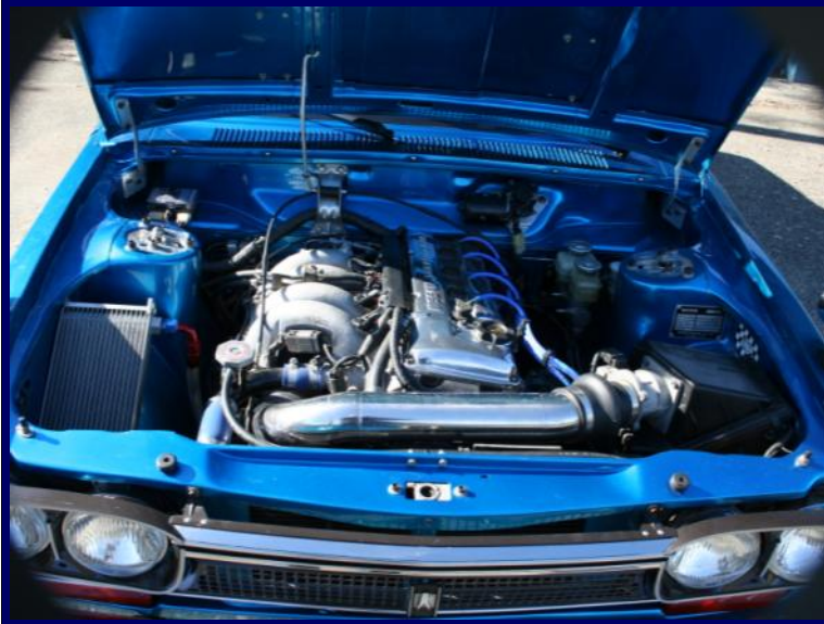
Photo 3—The worked KA24DE with oil cooler installation behind the right pair of headlights.
